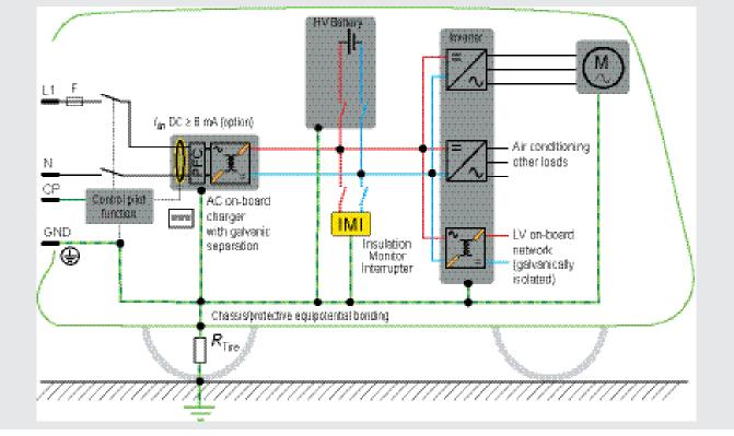
Insulation monitoring in an electric vehicle (EV) with an AC on-board charger with galvanic separation
