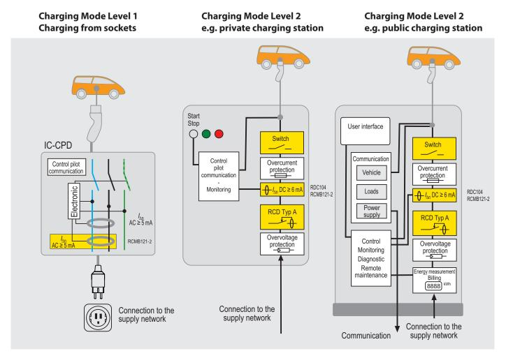
\* IC-CPD = In-Cable Control and Protective Device
