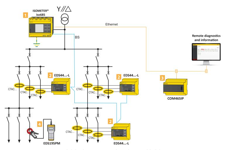
Figure 1: Ungrounded distribution system with Bender ground-fault location system.
